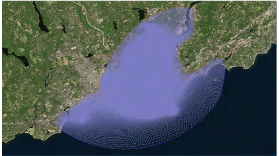
Figure 2.1 GZA High Resolution Computer Model Mesh
