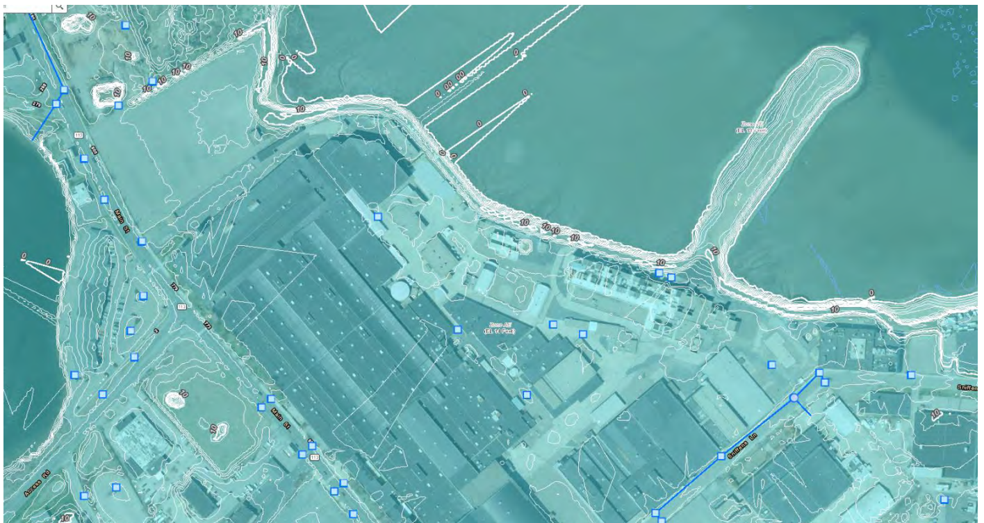
This figure indicates the effective FEMA FIRM limits of inundation and Base Flood Elevation. Existing storm drains, manholes and catch basins and area ground surface elevations also indicated.
