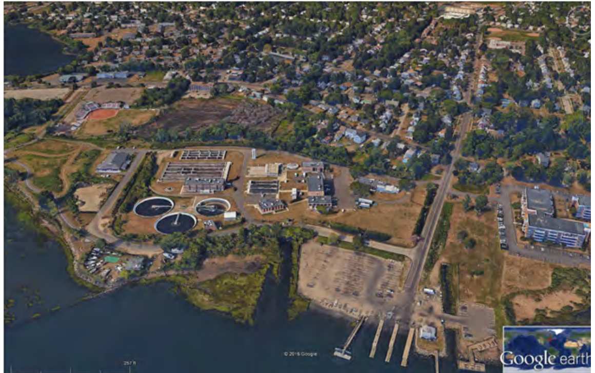
Image 18: The Stratford Wastewater Treatment Plant, including the plant’s discharge canal discharging to the Housatonic River. The plant is partially surrounded with a levee (perimeter roadway) with crest elevation of approximately Elevation 10 feet NAVD88. Image also shows the Birdseye Town Landing and boat ramp.
