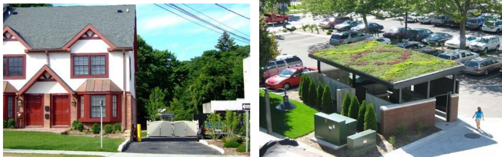
Refuse areas and mechanical equipment can be effectively screened with appropriate attention to design and materiality. The left image shows a refuse area designed to complement its attendant building. The
